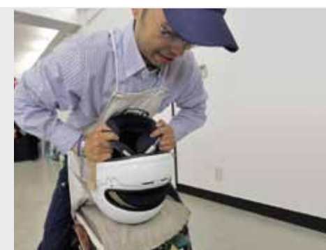
6 The inner shell is inserted into the outer shell – this can take a month of training to master
