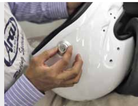
4 External components, like the HANS anchors can now be added on to the outer shell of the helmet
