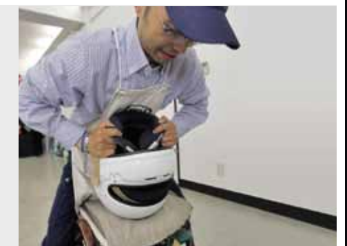
6 The inner shell is inserted into the outer shell – this can take a month of training to master
