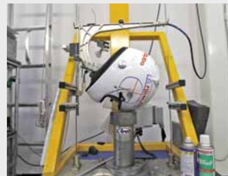
7 The finished helmet is subjected to punishing FIA tests to ensure that the optimum safety standard is achieved
